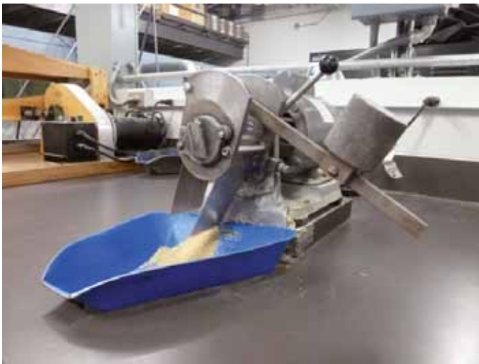
Photo 14-2. A laboratory-scale rice mill (McGill #2, Rapsco, Brookshire, Texas, USA).
