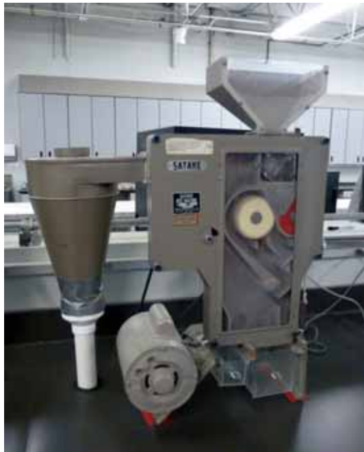
Photo 14-1. A laboratory-scale rice huller (THU 35B, Satake, Hiroshima, Japan).
