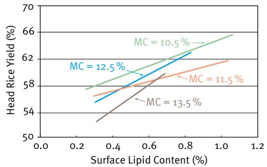
Fig. 5.5-2: Head rice yield vs. head rice surface lipid content for the CL XL745, long-grain cultivar milled at rough rice moisture contents of approximately 10.5%, 11.5%, 12.5%, and 13.5% (w. b.) for 10, 20, 30, and 40 s using a McGill #2 laboratory mill. Ref. 10
