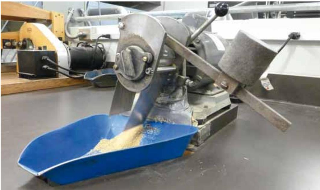
Fig. 5.4-1: McGill #2 laboratory-scale rice mill
