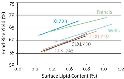
Fig. 5.5-1: Head rice yield vs. head rice surface lipid content of Wells, Francis, XL723, CL XL729, CL XL730, and CL XL745 cultivars milled at a rough rice moisture content of approximately 12.5% (w. b.) for 10, 20, 30, and 40 s using a McGill #2 laboratory mill. Source: Ref. 10
