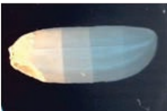
Photo 15-3. Illustration of a kernel fissured due to rapid moisture adsorption.
