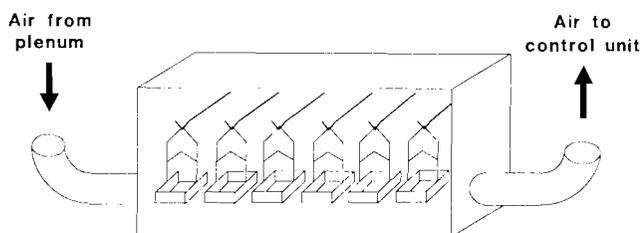
Figure 1—Conditioning chamber with tray locations and airflow directions.
