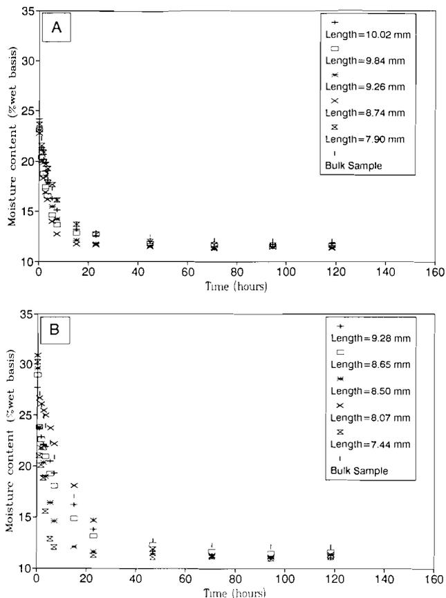
Figure 3—Drying data for long-grain rough rice kernels of various lengths for non-green (A) and green (B) kernels of the ‘Newbonnet’ variety. Air condition was 40° C and 60% RH.
