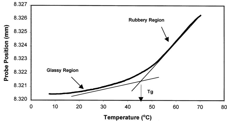
**Figure 1.** A typical thermal mechanical analysis thermogram indicating the assignment of the glass transition temperature ( $T_g$ ) and the glassy and rubbery region.
