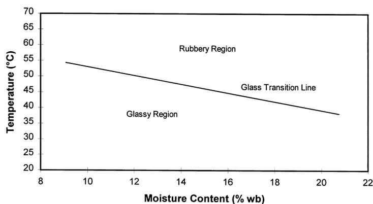
**Figure 2.** Combined state diagram for Bengal and Cypress indicating the glassy and the rubbery region.
