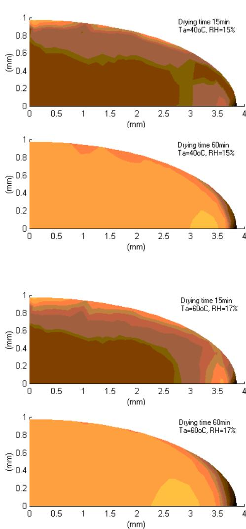
**Figure 4. Simulated radial stress ( $\sigma_{rr}$ ) distributions for a Cypress brown rice kernel (1/4 kernel shown) at initial moisture content of 20.0% (w.b.) and different drying stages ( $T_a$  = drying temperature, RH = drying air relative humidity). Positive and negative values are for tensile and compressive stresses, respectively.**
