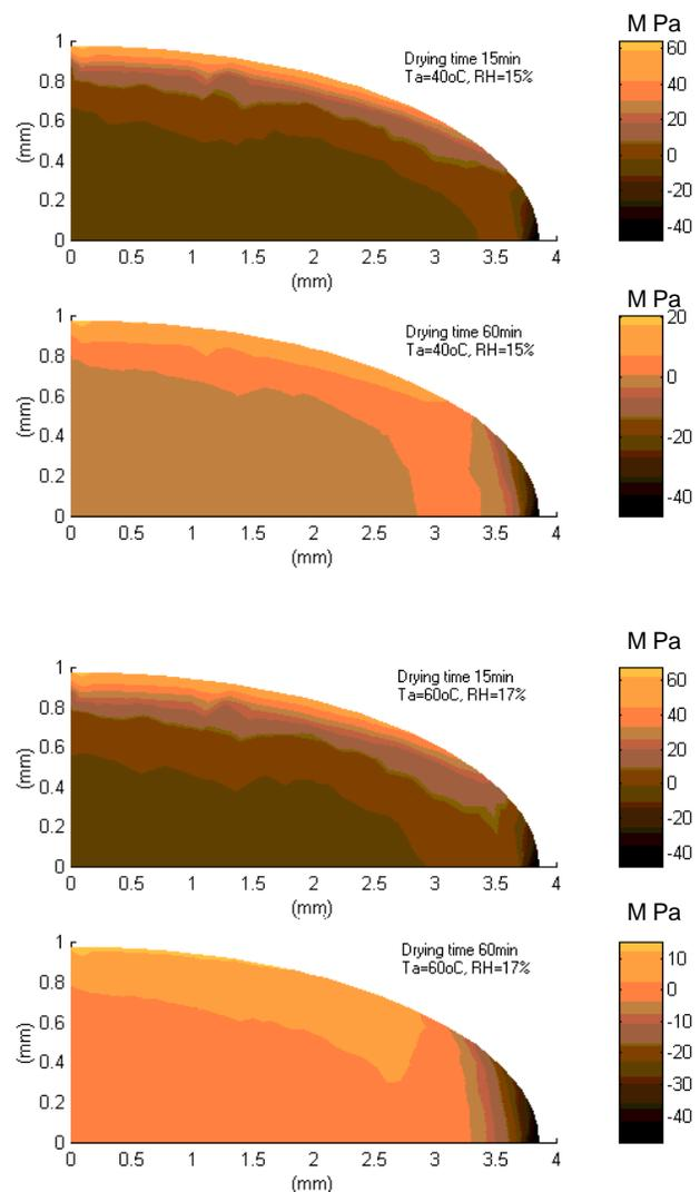
**Figure 5. Simulated axial stress ( $\sigma_{zz}$ ) distributions for a Cypress brown rice kernel (1/4 kernel shown) at initial moisture content of 20.0% (w.b.) and different drying stages ( $T_a$  = drying temperature, RH = drying air relative humidity). Positive and negative values are for tensile and compressive stresses, respectively.**
