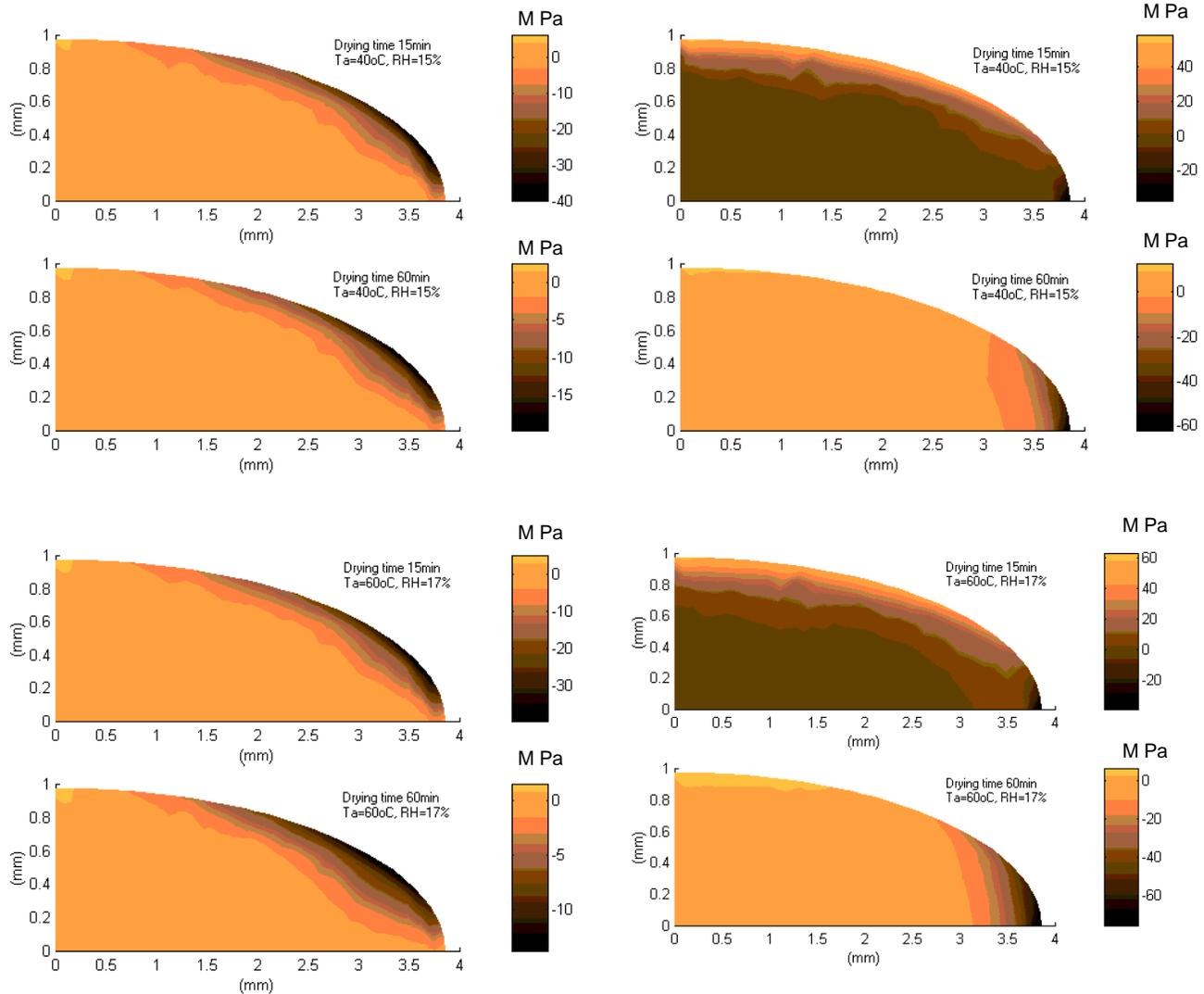
**Figure 6.** Simulated shear stress ( $\tau_{\theta z}$ ) distributions for a Cypress brown rice kernel (1/4 kernel shown) at initial moisture content of 20.0% (w.b.) and different drying stages ( $T_a$  = drying temperature, RH = drying air relative humidity). Positive and negative values are for tensile and compressive stresses, respectively.
