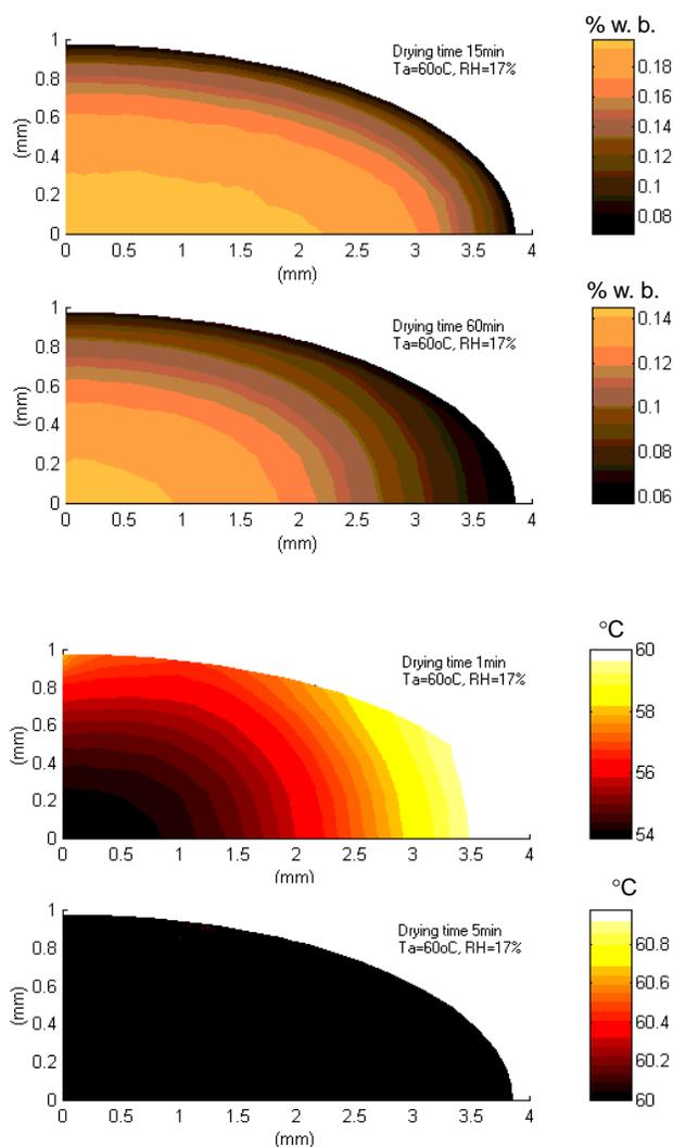
**Figure 3.** Moisture (upper two graphs) and temperature (lower two graphs) distributions at selected drying times for a Cypress brown rice kernel (1/4 kernel shown) at initial moisture content of 20.0% (w.b.) and equilibrium moisture content (EMC) of 6.0% (w.b.) ( $T_a$  = drying temperature, RH = drying air relative humidity).
