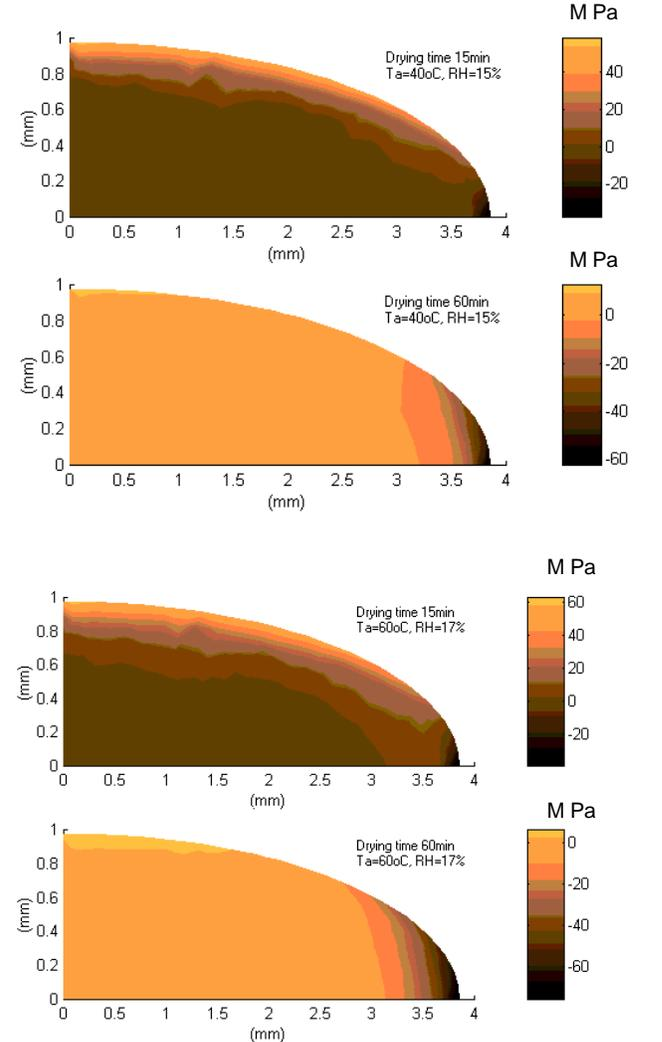
**Figure 7.** Simulated tangential stress ( $\sigma_{\theta\theta}$ ) distributions for a Cypress brown rice kernel (1/4 kernel shown) at initial moisture content of 20.0% (w.b.) and different drying stages ( $T_a$  = drying temperature, RH = drying air relative humidity). Positive and negative values are for tensile and compressive stresses, respectively.
