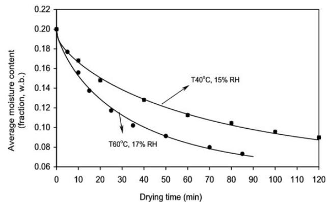
Figure 2. Simulated (curves) and measured (symbols) average moisture contents for a Cypress (long–grain) brown rice kernel at initial moisture content of 20.0% (w.b.) and two different drying conditions (T = drying temperature, RH = drying air relative humidity).
