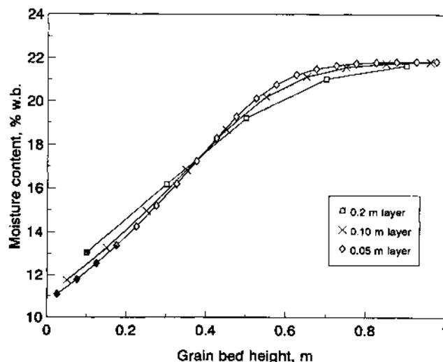
Figure 2—Moisture content profiles in a bed of rough rice when simulating with various layer thicknesses (initial m.c. 22.0% w.b.; bulk density  $550.2\text{ kg/m}^3$ ; air temperature  $30^\circ\text{C}$ ; RH 50%).
