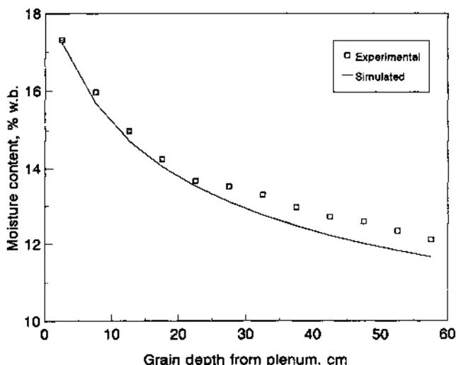
Figure 10—Experimental and simulated m.c. of rough rice in rewetting test no. 1 shown in table 2.
