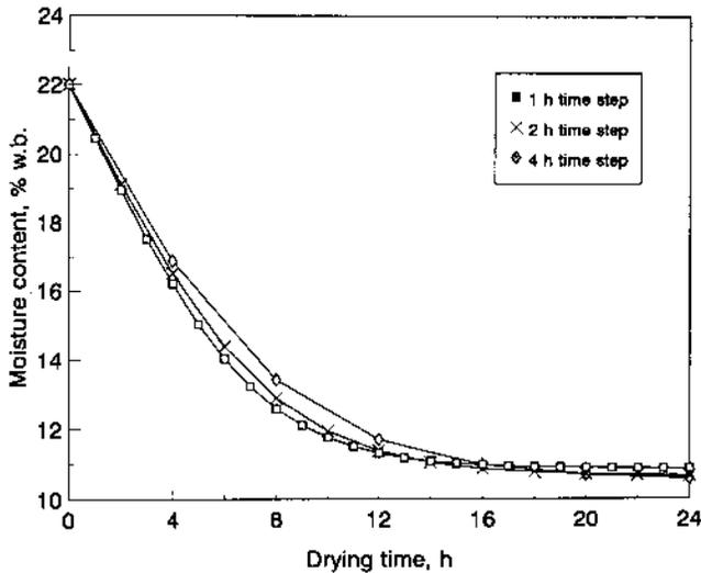
Figure 3—Simulated m.c. of a 0.1-m-thick layer of rough rice as a function of drying time step (Initial m.c. 22.0% w.b.; bulk density 550.2 kg/m<sup>3</sup>; air temperature 30° C; RH 50%; airflow rate 0.1 m<sup>3</sup>/s/m<sup>2</sup>).
