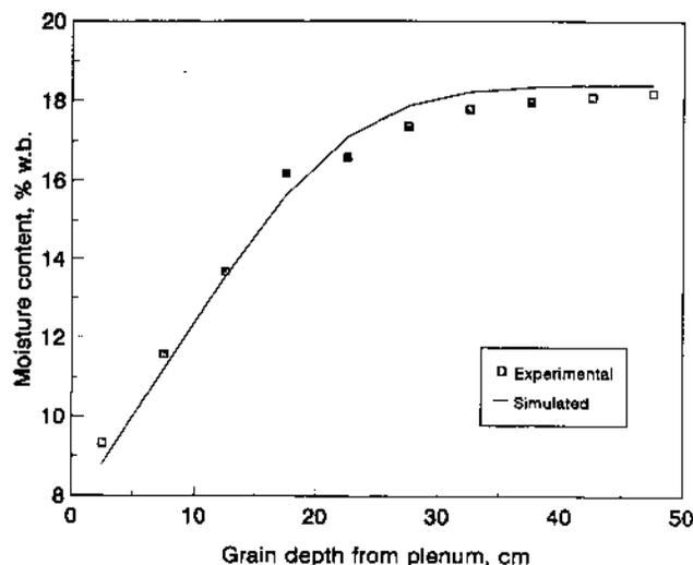
Figure 9—Experimental and simulated m.c. of rough rice in drying test no. 3 shown in table 2.
