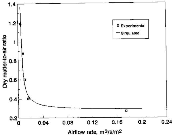
Figure 13—Relationship between grain dry matter-to-air ratio and air flow rate for drying and rewetting of rough rice in shallow beds (layer thickness 5 cm; time step 1 h).
