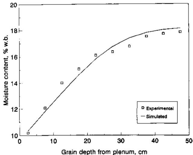
Figure 8—Experimental and simulated m.c. of rough rice in drying test no. 2 shown in table 2.
