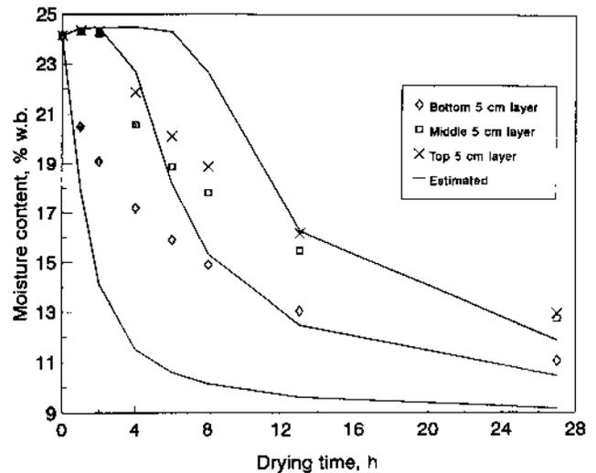
Figure 5—Experimental and simulated m.c. in multilayer drying of rough rice for conditions in test no. 1 shown in table 2.
