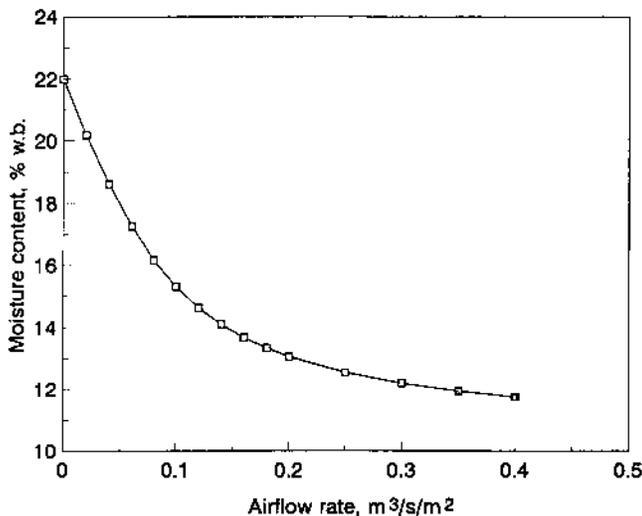
Figure 4—Simulated m.c. of a 0.1-m-thick layer of rough rice as a function of airflow rate (initial m.c. 22.0% w.b.; bulk density 550.2 kg/m<sup>3</sup>; air temperature 30° C; RH 50%; drying time step 1 h).
