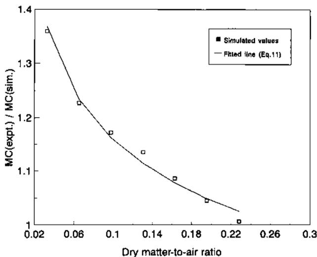
Figure 7—Average values of the ratio of experimental to simulated m.c. of rough rice as a function of dry matter-to-air ratio based on a 1-h time step in multilayer drying test no. 1 shown in table 2. Dry matter-to-air ratio was varied by progressively combining grain layers.
