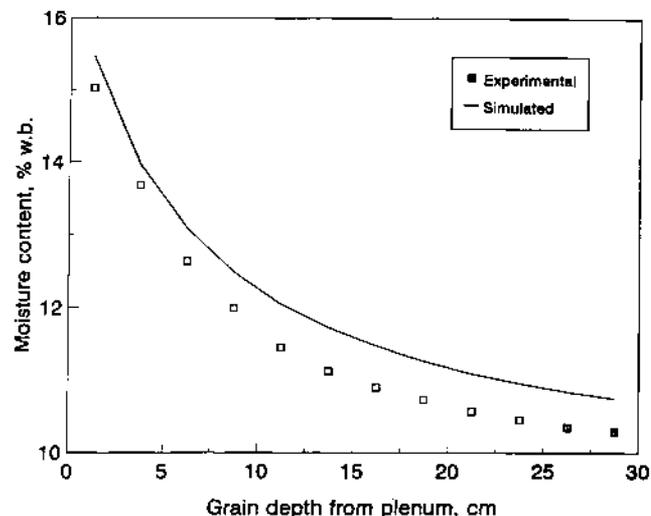
Figure 11—Experimental and simulated m.c. of rough rice in rewetting test no. 2 shown in table 2.
