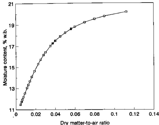
Figure 1—Simulated m.c. of a 0.1-m-thick layer of rough rice as a function of dry matter-to-air ratio (initial m.c. 22.0% w.b.; bulk density  $550.2\text{ kg/m}^3$ ; air temperature  $30^\circ\text{C}$ ; RH 50%).
