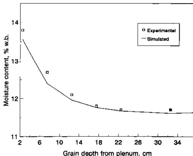
Figure 12—Experimental and simulated m.c. of rough rice in rewetting test no. 3 shown in table 2.
