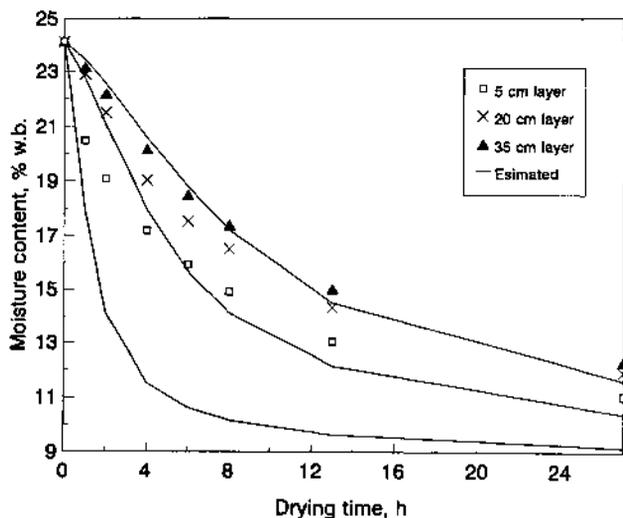
Figure 6—Experimental and simulated m.c. of rough rice in test no. 2 shown in table 2 when selected layers were combined.
