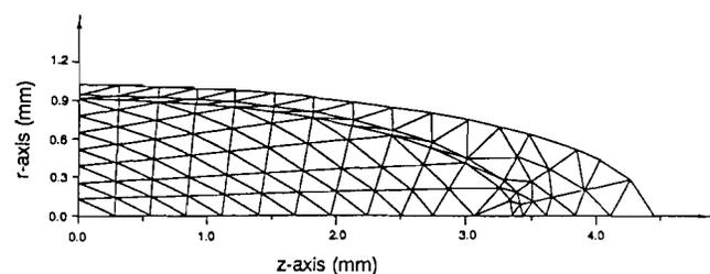
Figure 2—Finite element grid for an axisymmetric model of a long-grain rough rice kernel (108 nodes, 172 elements).
