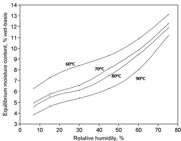
Figure 4. Equilibrium moisture contents (%, wet basis), determined as asymptotic values of the Page equation (eq. 3) for Cybonnett rice samples dried at 60°C to 90°C and 7% to 75% RH in a fluidized-bed system. Each data point is an average of three replications.
