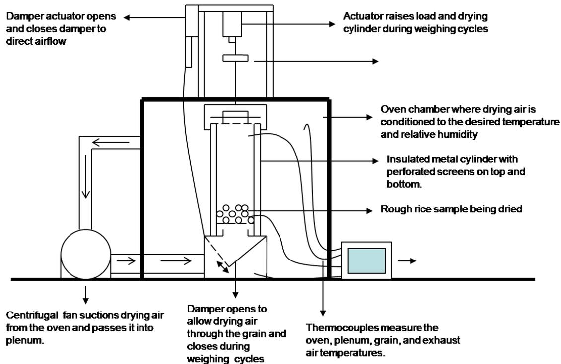
Figure 1. Schematic of the high-temperature, fluidized-bed drying system.
