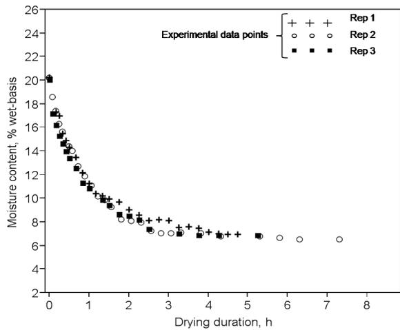
Figure 2. Fluidized-bed drying data for Cybonnett rice samples dried at 60°C and 7% RH.
