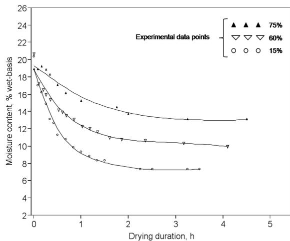
Figure 3. Fluidized-bed drying data for Cybonnett rice samples dried at 60°C and 15%, 60%, and 75% RH. The solid lines illustrate trends in the drying data.
