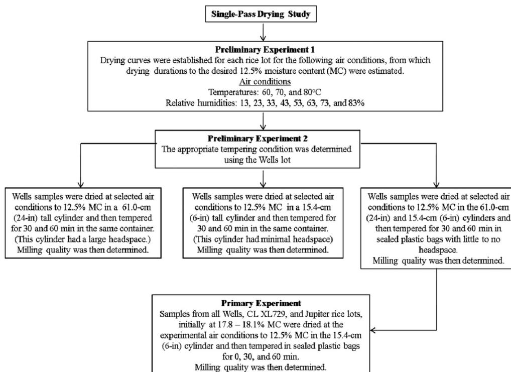
FIG. 2. Experimental design of the single-pass drying study. The drying characteristics and milling quality of pure-line long-grain Wells and hybrid CL XL729, and pure-line medium-grain Jupiter initially at 17.8–18.1% moisture content was investigated.
