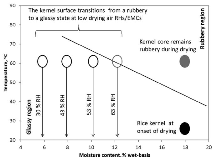
FIG. 1. Hypothetical material state differences between the surface and the core of a rice kernel caused by the relative humidity (RH)/equilibrium moisture content (EMC) associated with the drying air. The glass transition diagram was taken from Siebenmorgen et al.<sup>[4]</sup>
