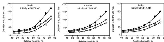
FIG. 4. Drying times required to attain 12.5% moisture content (MC) for Wells, CL XL729, and Jupiter rice samples, initially at 17.8–18.1% MC, dried at (●) 60°C, (□) 70°C, and (○) 80°C and 13–83% relative humidity. The drying durations were estimated from drying curves.
