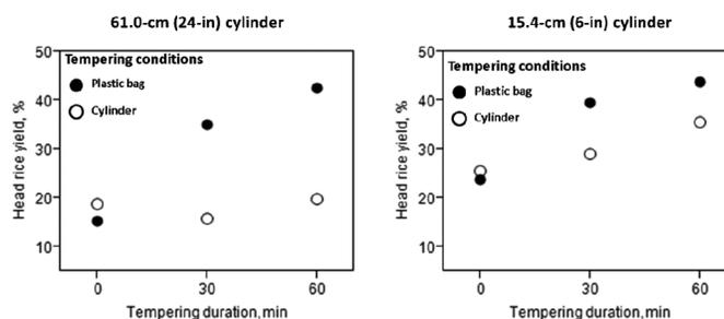
FIG. 5. Head rice yields of Wells samples dried at 70°C and 13% relative humidity to 12.5% moisture content in a single pass in either the 61.0-cm (24-in.) or 15.4-cm (6-in.) cylinder and then tempered in the 61.0-cm (large headspace) or 15.4-cm (small headspace) cylinder or a sealed plastic bag (minimal headspace). Data points are an average of four measurements; that is, two replications with each replicate head rice yield measured in duplicate. The head rice yield of the control was 51.2%.
