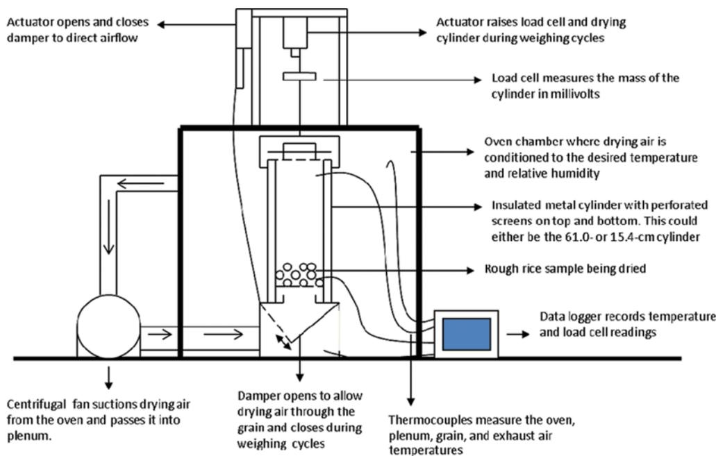
FIG. 3. Schematic of the fluidized bed drying system (color figure available online).
