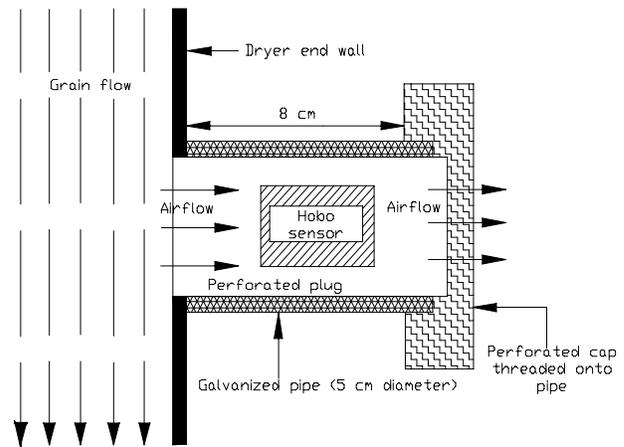
**Figure 4.** Schematic of a sampling port that was used to house an air temperature and relative humidity sensor and that allowed rice to be removed for moisture content and head rice yield determination.
