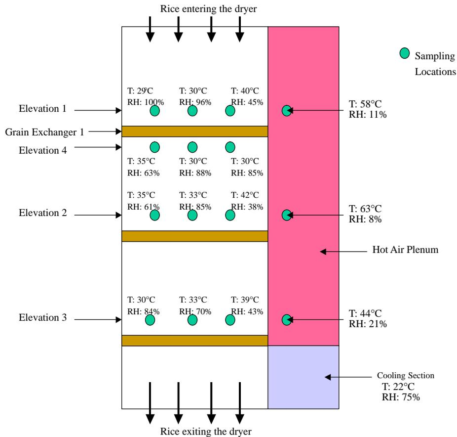
Figure 7. Air temperature (T) and relative humidity (RH) data for various locations within the cross-flow dryer at 12:00 A.M. for the 11 September 2002 testing run. RHs reported in the hot air plenum were estimated using air inlet temperature and RH.
