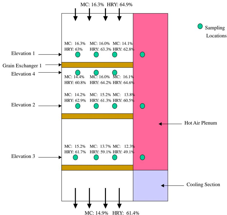
Figure 8. Moisture content (MC) and head rice yield (HRY) data for various locations within the cross-flow dryer at the end of the 11 September 2002 testing run.
