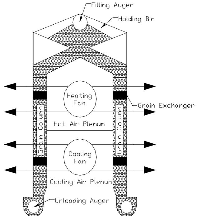
Figure 1. Schematic of a commercial cross-flow dryer adapted from Brooker et al. (1992).
