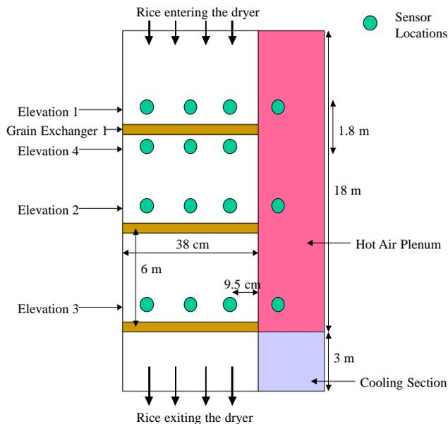
**Figure 3.** Design layout for the temperature and relative humidity sensor locations in the cross-flow rice dryer for the year 2001 and 2002 test runs. Elevation 4 was later added in the 2002 test runs to determine grain exchanger effects.
