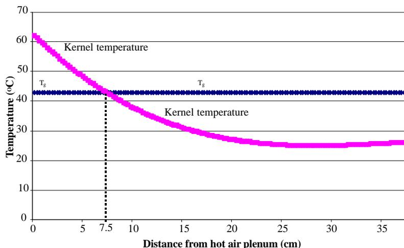
Figure 9. Illustration of an extreme drying case measured on 26 September 2001 in which rice located between the hot air plenum and 7.5 cm inside the rice column at elevation 1 exceeded glass transition temperature ( $T_g$ ). A constant  $T_g$  of 43°C was calculated based on incoming moisture content of 17.8% according to figure 2.
