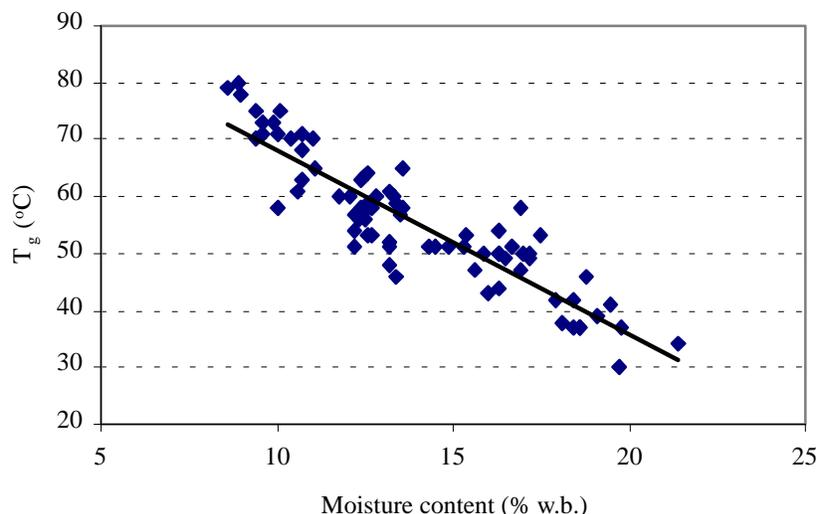
Figure 2. Glass transition temperature ( $T_g$ ) for long-grain rice as reported by Siebenmorgen et al. (2004).
