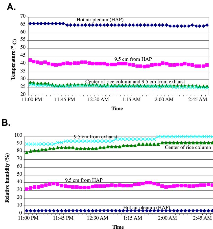
Figure 5. Air temperature (A) and relative humidity (B) history at elevation 1 (fig. 3) during the 1 October 2001 test run. The relative humidity in the HAP (4%) was estimated based on the air inlet temperature and relative humidity.
