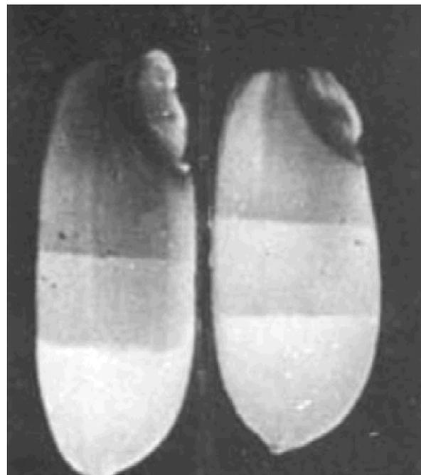
**Figure 2. Images of rice kernels fissured after drying at 60° C and 17% RH for 40 min and then exposed to ambient air. The images were obtained with a video microscopy system (Bautista et al., 2000).**
