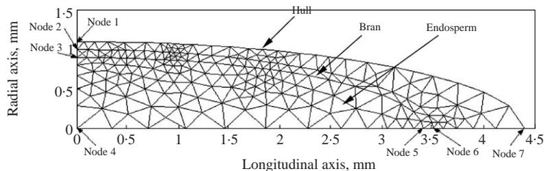
Fig. 1. Finite element mesh of a long-grain rough rice kernel (variety Cypress,  $\frac{1}{4}$  section)
