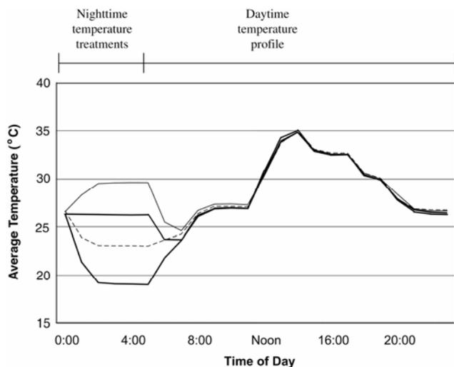
**Fig. 1.** Measured temperature profiles within the phytotrons. Each profile was obtained by averaging, at 2-hr intervals, the actual air temperature from two canopy-height temperature sensors over the study duration.
