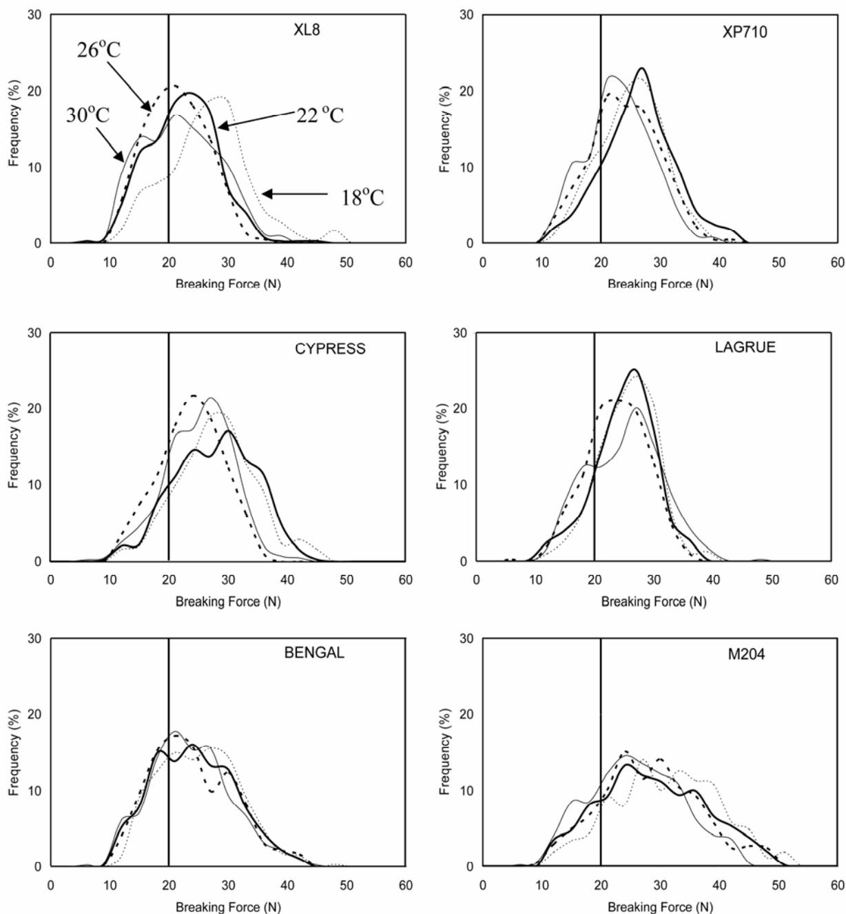
**Fig. 4.** Breaking force distributions of indicated cultivars grown at 18, 22, 26, and 30°C nighttime air temperatures determined through three-point bending tests (two replicates of 200 brown rice kernels). Brown rice kernels requiring a force >20 N to break were classified as “strong” kernels and correlated with adjusted head rice yield (Fig. 5).
