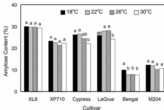
Fig. 7. Milled rice amylose content of indicated cultivars grown at 18, 22, 26, and 30°C nighttime air temperatures. Each data point represents the average of two replicates for which measurements were performed in duplicate. Means within each cultivar group with the same letter were not significantly ( $P > 0.05$ ) different.
