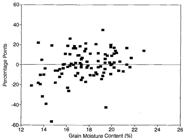
**Figure 1—Difference between loss rates calculated using grain yields from a commercial combine and loss rates calculated using grain yields from a plot combine for tests conducted in 'Newbonnet' and 'Lemont' rice in 1990.**
