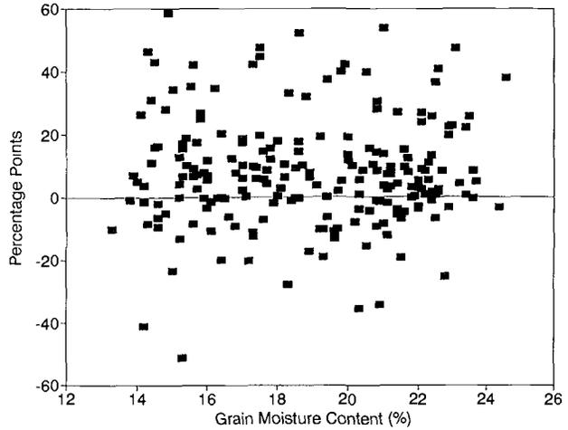
**Figure 2—Difference between loss rates calculated using grain yields from a commercial combine and loss rates calculated using grain yields from a plot combine for tests conducted in 'Newbonnet' and 'Lemont' rice in 1991.**
