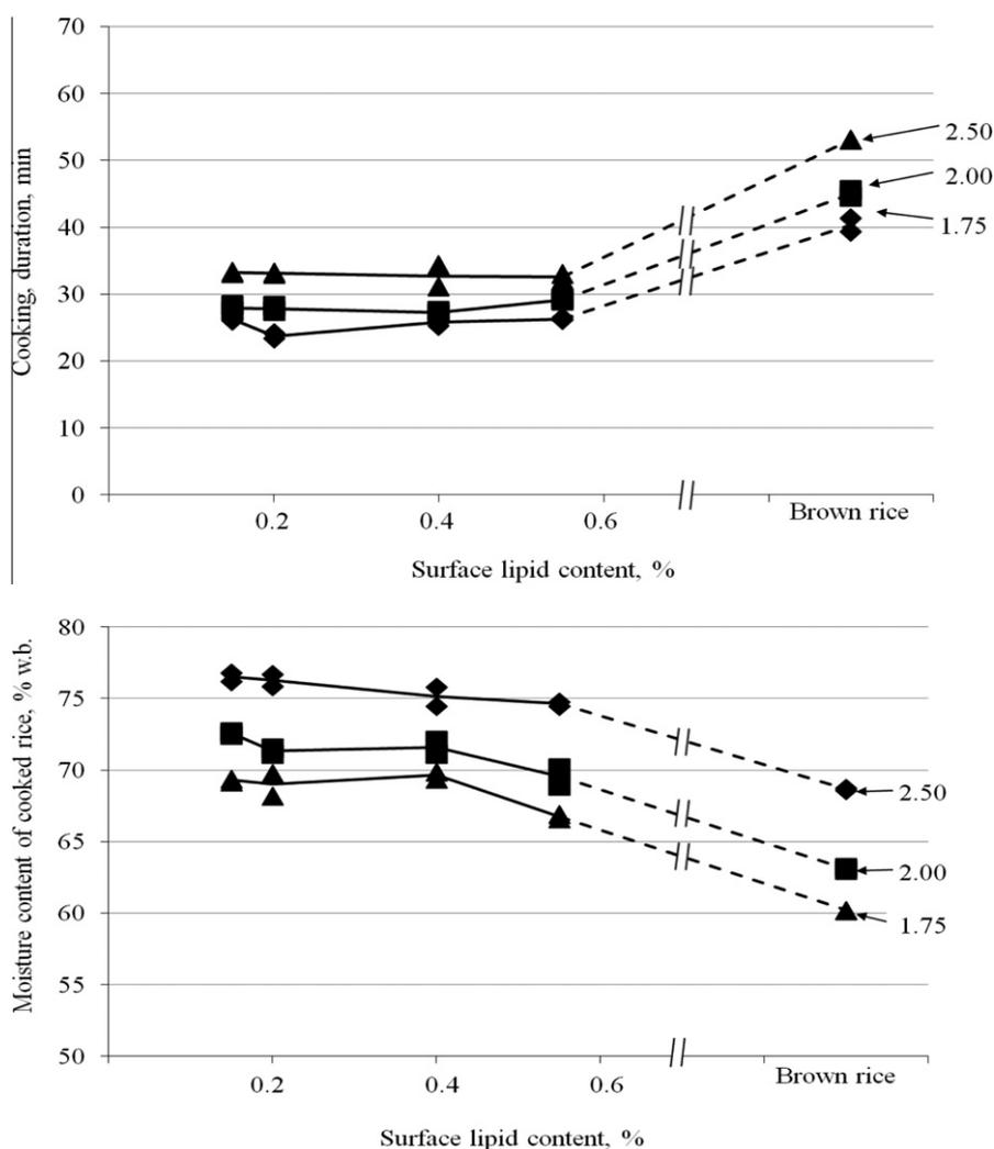
**Fig. 2.** Cooking duration and moisture content of non-parboiled rice with the indicated SLCs that was cooked in a rice cooker using 1.75, 2.00 and 2.50 water-to-rice ratios. Data points indicate either cooking duration measured at the end of each cooking replication or the mean of three duplications of moisture content at the end of each cooking replication.
