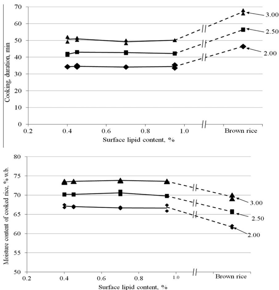
**Fig. 4.** Cooking duration and moisture content of parboiled rice with the indicated surface lipid contents that was cooked in a rice cooker using 2.00, 2.50 and 3.00 water-to-rice ratios. Data points indicate either cooking duration measured at the end of each cooking replication or the mean of three duplications of moisture content at the end of each cooking replication.
