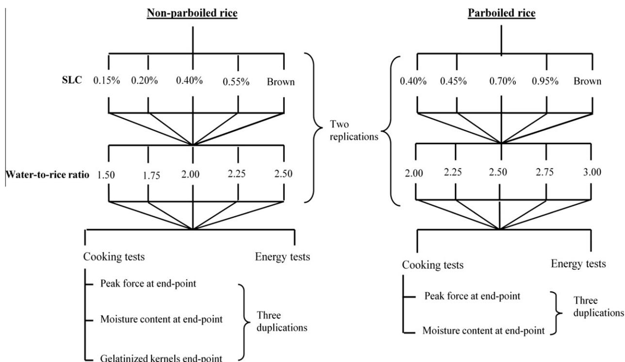
Fig. 1. Experimental design for tests in which rice was cooked under controlled water-to-rice mass ratios.
