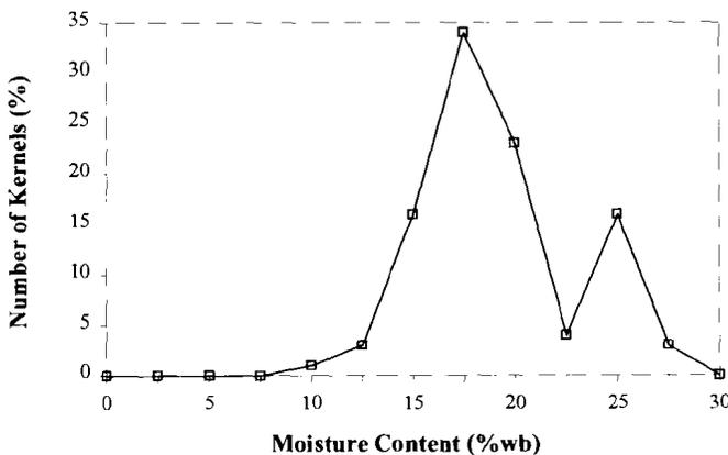
**Fig. 1.** Kernel moisture content distribution for cultivar Cypress long-grain rice harvested at 19.2% wb. The bimodal moisture content distribution is a characteristic of rough rice at harvest.
