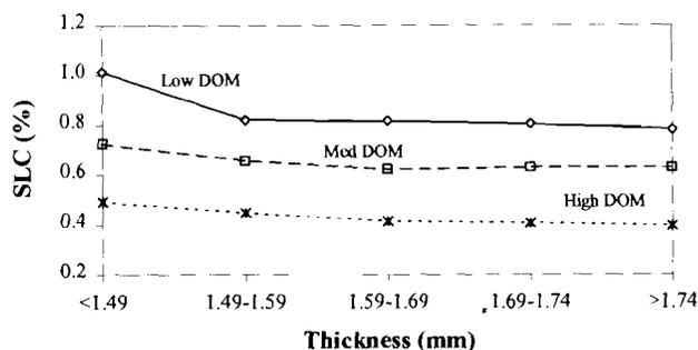
**Fig. 3.** Surface lipid concentrations (SLCs) of different thickness fractions vary within a bulk sample milled to different degree-of-milling (DOM) levels. The thinner kernels are not milled to the same SLC as the thicker kernels at the lower DOM levels.
