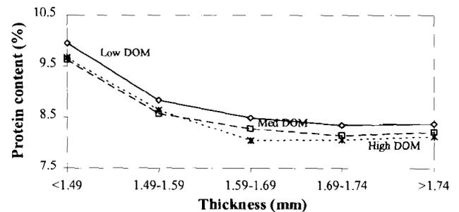
**Fig. 4.** Protein content of different thickness fractions vary within bulk samples of milled rice that were milled to different degree-of-milling (DOM) levels. After milling, the thinner kernels have significantly higher protein contents than other thickness fractions.
