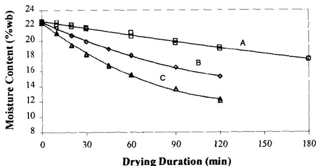
**Fig. 5.** Moisture content curves resulting from drying cultivar Bengal medium-grain rice at conditions A (43°C, 38% rh), B (52°C, 25% rh), and C (60°C, 17% rh).
