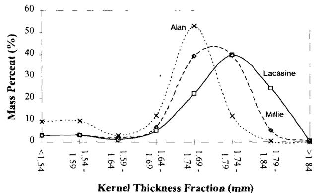
**Fig. 2.** Mass distributions of head rice kernel thickness fractions for three long-grain cultivars reflect the natural variability present within a bulk sample.
