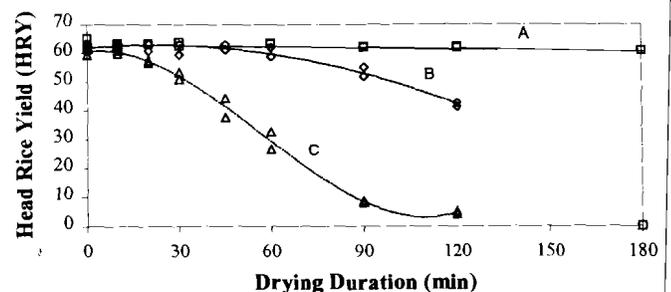
**Fig. 6.** Head rice yield curves corresponding to the drying durations and conditions given in Fig. 5.
