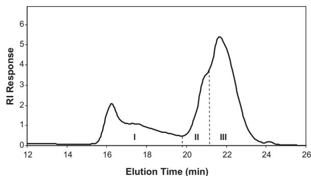
**Figure 2.** Chromatogram of debranched starch (I, AM; II, long AP chain; III, short AP chain)
