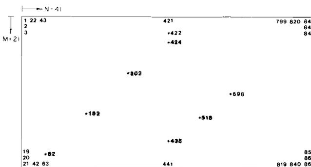
Figure 1-Cross-section of a bunker storage unit with grid orientation. Grid consisted of 41 points (N) in the x-direction and 21 points (M) in the y-direction.
