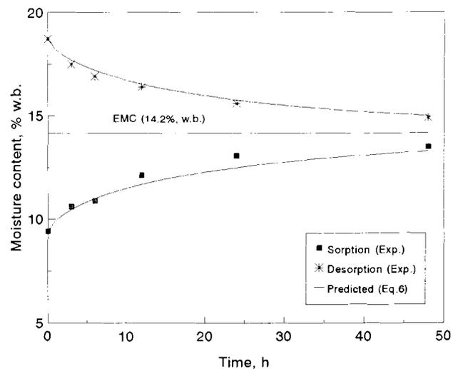
Figure 7—Comparison of experimental and predicted MCs of rough rice during moisture desorption and sorption tests.
