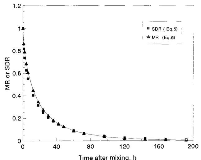
Figure 8—Relative comparison of changes in SD ratio and moisture ratio with time in blended rough rice.
