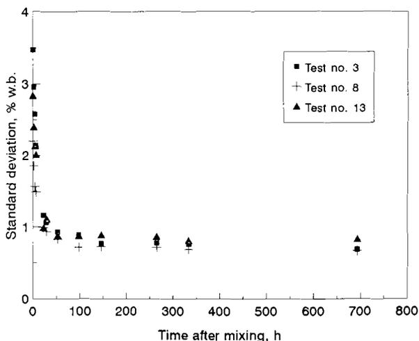
Figure 3—SD of MCs in blended rough rice as a function of time for mixing condition shown in table 1.
