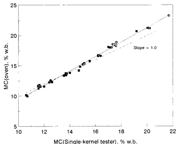
Figure 1—Comparison of rough rice MCs based on bulk sample oven determinations and single-kernel moisture tester measurements.
