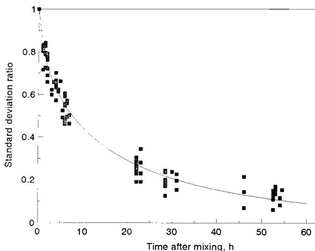
Figure 5–The SD ratio of blended rough rice as a function of time.
