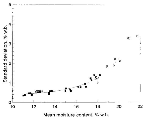
Figure 2—Relationship between SD of individual kernel MCs and mean MC of rough rice determined with the single-kernel moisture tester.
