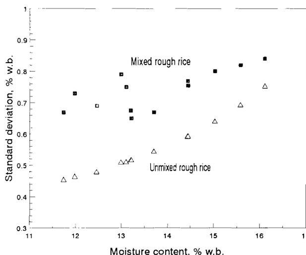
Figure 4—Comparison of SD of MCs in blended rough rice with that of unmixed rough rice at the mean MC of the mixture.
