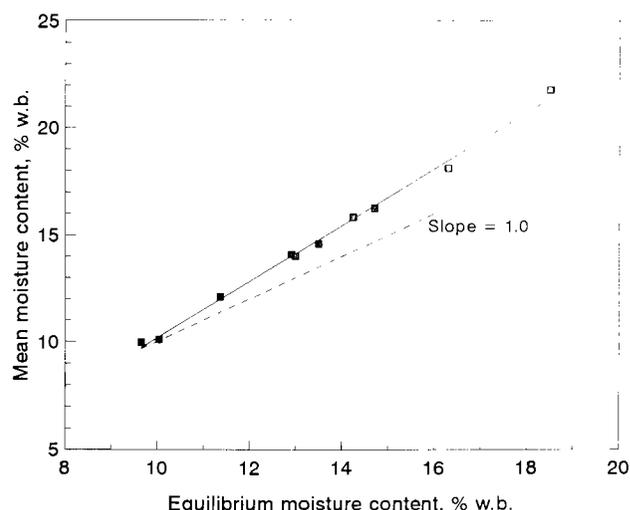
Figure 6–Relationship between mean MC of blended rough rice and EMC estimated by the Chung equation.
