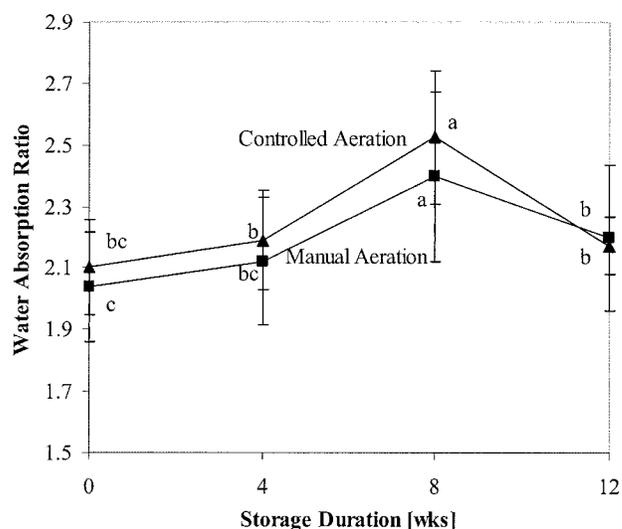
**Fig. 1.** Water absorption ratio of cooked rice as a function of storage duration for manual aeration and controlled aeration. Error bars show ± standard deviation. Values with the same letter are not significantly different at  $P < 0.05$ .
