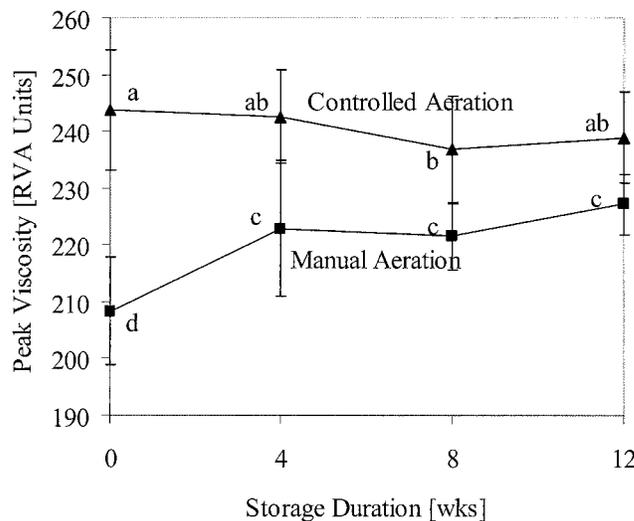
**Fig. 2.** Peak viscosity values of rice slurries as a function of storage duration for manual aeration and controlled aeration. Error bars show ± standard deviation. Values with the same letter are not significantly different at  $P < 0.05$ .
