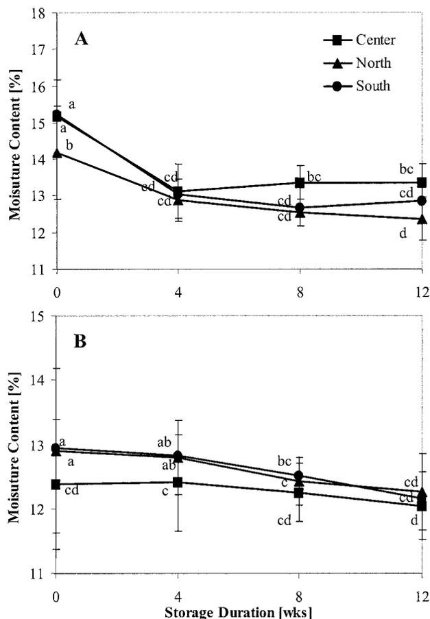
**Fig. 3.** Moisture content (MC) of rough rice as a function of storage duration and bin sample location for manual aeration (A) and controlled aeration (B). Average standard deviation was 0.27%. Values with the same letter in each graph are not significantly different at  $P < 0.05$ .
