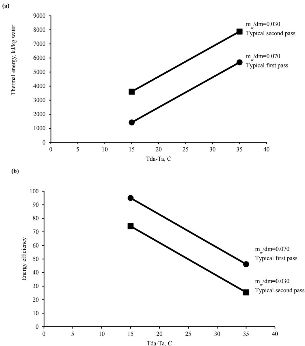
Figure 7. Family of curves predicting thermal energy use (a) and thermal energy efficiency (B) as a function of the difference between drying air temperature and ambient temperature ( $T_{\text{da}} - T_a$ ) at the indicated levels of water removed per mass dry matter ( $m_w/dm$ ) for drying tests conducted in 2011 and 2012. Drying air temperatures ranged from 45°C to 55°C and ambient air temperatures ranged from 15°C to 30°C.
