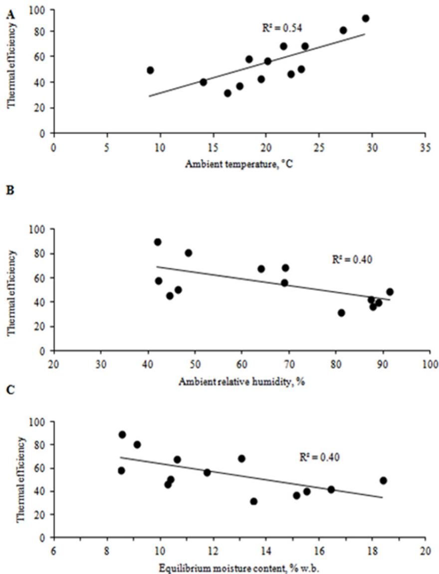
Figure 6. Thermal energy efficiency per drying run, calculated as the ratio of theoretical energy requirements ( $E_{\text{theo}}$ ) divided by the measured thermal energy ( $E_{\text{thermal}}$ ), of the on-farm dryer as a function of average ambient temperature (a), average ambient relative humidity (b) and rough rice equilibrium moisture content associated with the ambient air temperature and relative humidity predicted by the Chung-Pfost equation (c).
