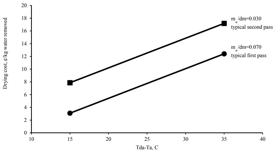
Figure 8. Family of curves predicting drying cost as a function of the difference between drying air temperature and ambient temperature ( $T_{\text{da}} - T_a$ ) at the indicated levels of water removed per mass dry matter ( $m_w/dm$ ) for drying tests conducted in 2011 and 2012. Drying air temperatures ranged from 45°C to 55°C and ambient air temperatures ranged from 15°C to 30°C.
