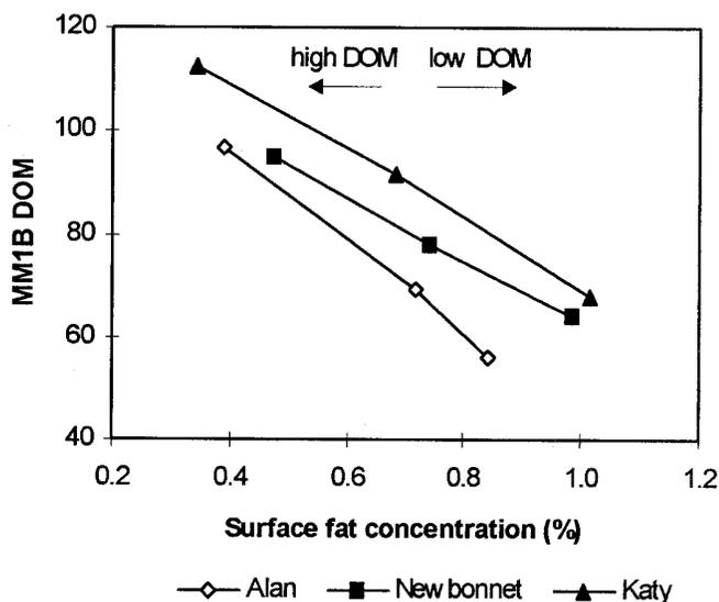
Fig. 3. Degree of milling (DOM) as measured by a Satake MM1B milling meter vs. surface fat concentration of unfractionated head rice for each of the indicated long-grain cultivars. Each point represents an average of duplicate measurements.
