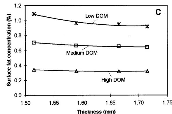
Fig. 5. Surface fat concentration (SFC) of milled rice kernel thickness fractions at three degree of milling (DOM) levels for cultivars Alan (A), Newbonnet (B), and Katy (C) milled as an unfractionated bulk. Each point is an average of two SFC determinations.
