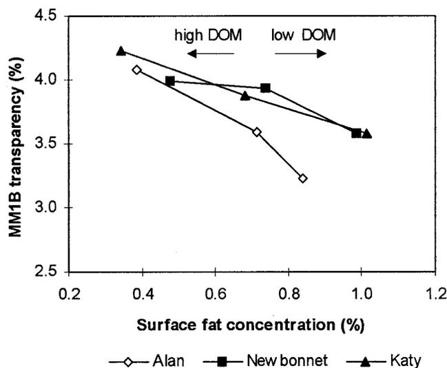
Fig. 2. Transparency as measured by a Satake MM1B milling meter vs. surface fat concentration of unfractionated head rice for each of the indicated long-grain cultivars. Each point represents an average of duplicate measurements.
