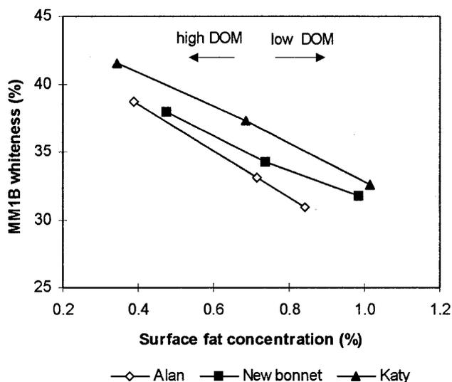
Fig. 1. Whiteness as measured by a Satake MM1B milling meter vs. surface fat concentration of unfractionated head rice for each of the indicated long-grain cultivars. Each point represents an average of duplicate measurements.
