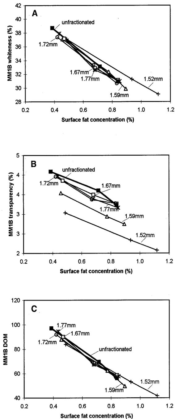
Fig. 6. Whiteness (A), transparency (B), and degree of milling (DOM) (C) as measured by a Satake MM1B milling meter vs. surface fat concentration for unfractionated head rice and various milled rice kernel thickness fractions of Alan.
