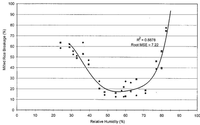
**Fig. 1.** Medium-grain milled rice kernel breakage resulting from 20 min of exposure to air at 30°C and 25–82% RH at a constant rough rice kernel moisture content of 12.5% (wb). Trendline used a best-fit polynomial. Each data point represents average of two replicates (◆ = Bengal, ■ = Orion).
