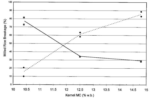
**Fig. 2.** Medium-grain rice (Bengal) kernel breakage resulting from 20 min of exposure to air environments of high and low relative humidities (30°C, 75% RH [■]) (30°C, 23% RH [◆]) over a range of rough rice moisture contents.
