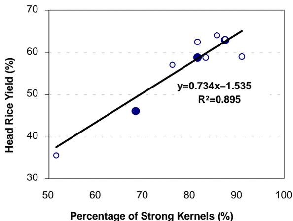
Figure 7. Percentage of “strong” kernels (kernels withstanding a 20 N force in a three-point bending test) vs. head rice yield. Darkened data symbols represent the first three entries in table 1, while open symbols represent the other seven samples tested.
