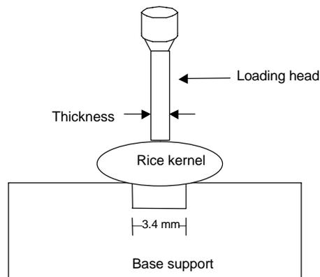
Figure 1. Schematic of the three-point bending test device. The loading head was 1.48 mm thick and 9.9 mm wide with a flat surface.
