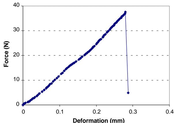
Figure 2. Typical force–deformation curve for a brown rice kernel under three–point bending.
