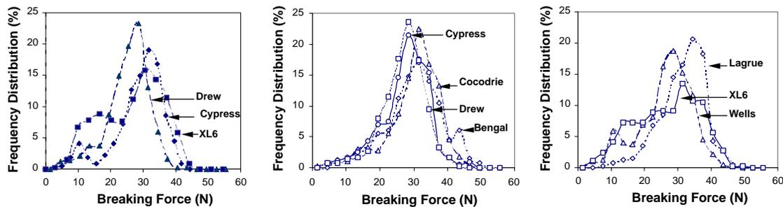
Figure 6. Breaking force distributions for the brown rice samples listed in table 1. Darkened data symbols represent the first three entries, while open symbols represent the other seven samples tested.
