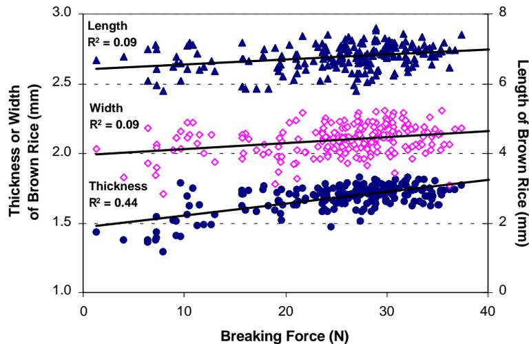
Figure 4. Physical dimensions vs. breaking force of Cypress brown rice kernels.
