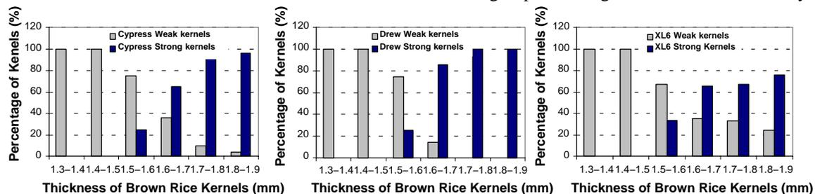
Figure 5. Percentage of “weak” and “strong” brown rice kernels in different thickness fractions of Cypress, Drew, and XL6 brown rice kernels. Strong kernels were those withstanding greater than a 20 N force in a three-point bending test.
