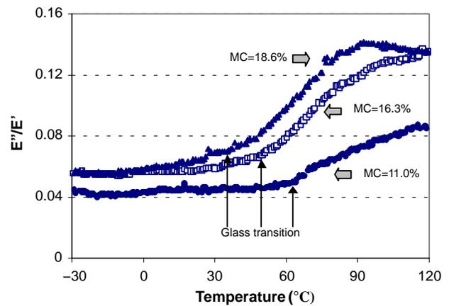
**Figure 2.** The effect of moisture content (w.b.) on the spectra of  $E''/E'$  vs. temperature for brown rice kernels (cv. Bengal).
