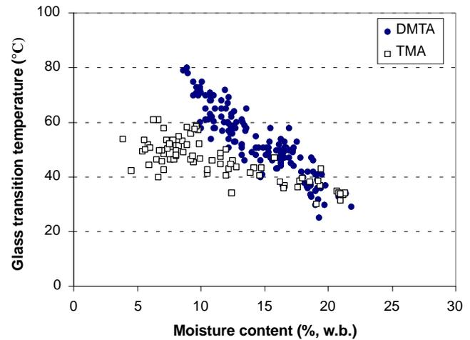
Figure 4. Comparison of glass transition temperatures of brown rice kernels measured using dynamic mechanical thermal analysis (DMTA, data from fig. 3) and thermal mechanical analysis (TMA, Sun et al., 2002).
