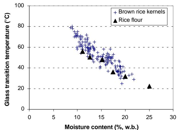
Figure 5. Comparison of glass transition temperatures of brown rice kernels measured using dynamic mechanical thermal analysis (data from fig. 3) with those of rice flour as determined using a phase transition analyzer (Plattner, 2001).
