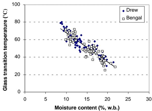
Figure 3. Glass transition temperature vs. moisture content for Drew and Bengal brown rice kernels as determined by dynamic mechanical thermal analysis.
