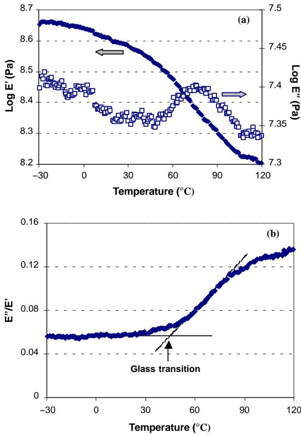
**Figure 1.** Dynamic mechanical thermal analysis curves for a brown rice kernel (cv. Bengal) at 16.3% moisture content: (a) temperature dependence of the storage modulus ( $E'$ ) and the loss modulus ( $E''$ ), and (b) temperature dependence of  $E''/E'$ .
