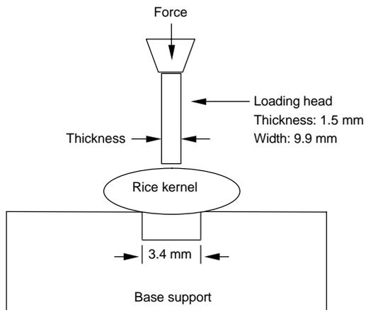
Figure 1. Schematic of the three-point bending test device.
