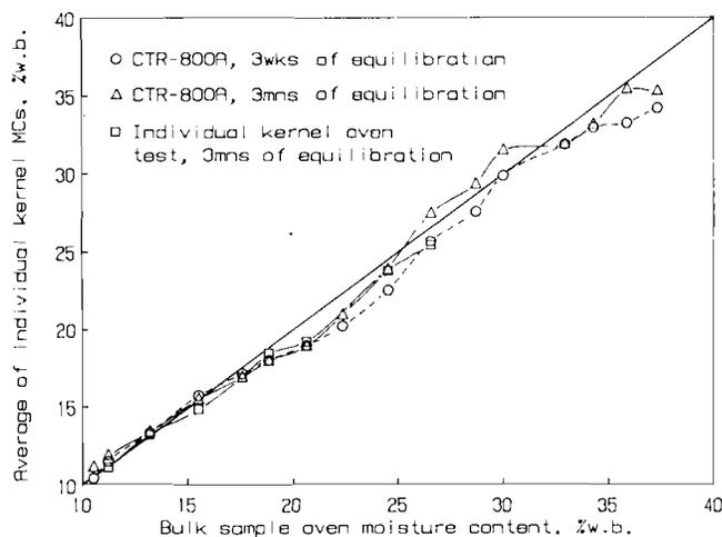
**Figure 1—Comparison of average MCs determined after three weeks and three months of equilibration using a Shizuoka Seiki CTR-800A moisture meter to those measured with an individual kernel oven method and a bulk sample oven method.**
