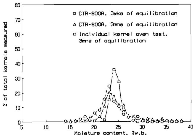
Figure 3—Individual kernel MC frequency distributions for a low and high MC sample as measured after three weeks and three months of equilibration using a Shizuoka Seiki CTR-800A moisture meter and an individual kernel oven method.
