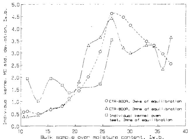
**Figure 2—Average individual kernel MC standard deviations determined from MC data taken after three weeks and three months of equilibration using a Shizuoka Seiki CTR-800A moisture meter and an individual kernel oven method.**
