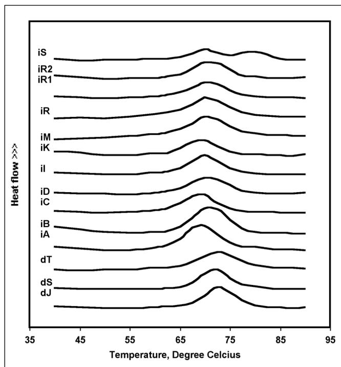
**Figure 1—Gelatinization properties of jasmine rice samples using differential scanning calorimetry (DSC). Sample abbreviations can be found in Table 1.**
