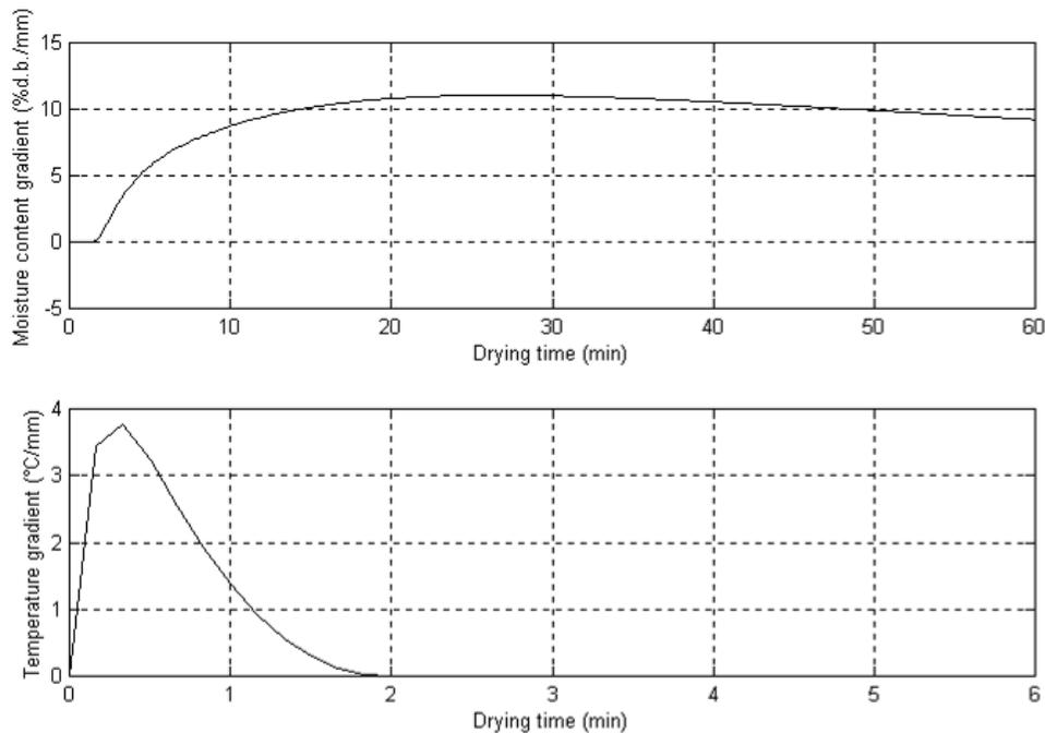
Figure 5. MCGs between node 2 and node 4 and temperature gradients between node 4 and node 6 in figure 1 at 60° C drying air temperature and 17% air relative humidity.
