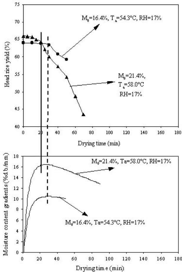
Figure 6. An illustration showing the time when head rice yield started to drop dramatically in the case of no tempering performed on rice after drying coincided with the time around which MCG peaked (redrawn from the data reported by Yang et al., 2000a.)
