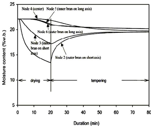
Figure 8. A graph showing the way the estimated moisture content at five specified nodes of a rough rice kernel (22.1% w.b. initial moisture content) changes during the drying and the subsequent adiabatic tempering process. The drying condition was 60° C and 17% relative humidity, and adiabatic tempering was conducted at 60° C.
