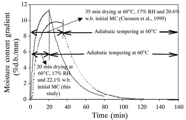
Figure 7. A graph showing the MCGs during drying at 60°C and 17% relative humidity for 20 min and 35 min, respectively, and the subsequent adiabatic tempering at 60°C. The data for 20 min drying were collected in this study with rice at 22.1% w.b. initial moisture content and those for 35 min drying were based on Cnossen et al. (1999) with rice at 20.6% w.b. initial moisture content.
