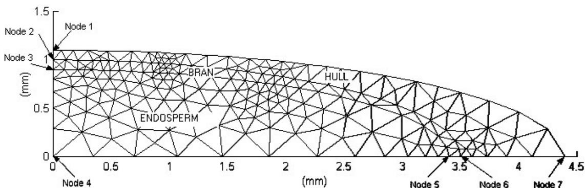
Figure 1. Finite element mesh of a long-grain (cv. Cypress) rice kernel (1/4 section).
