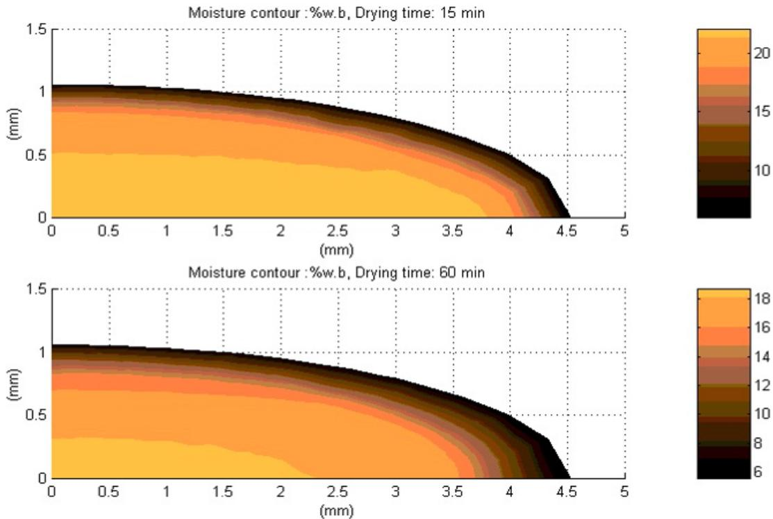
Figure 4. Simulated moisture content distribution inside a rough rice kernel (22.1% w.b. initial moisture content) under 60° C drying air temperature and 17% air relative humidity.
