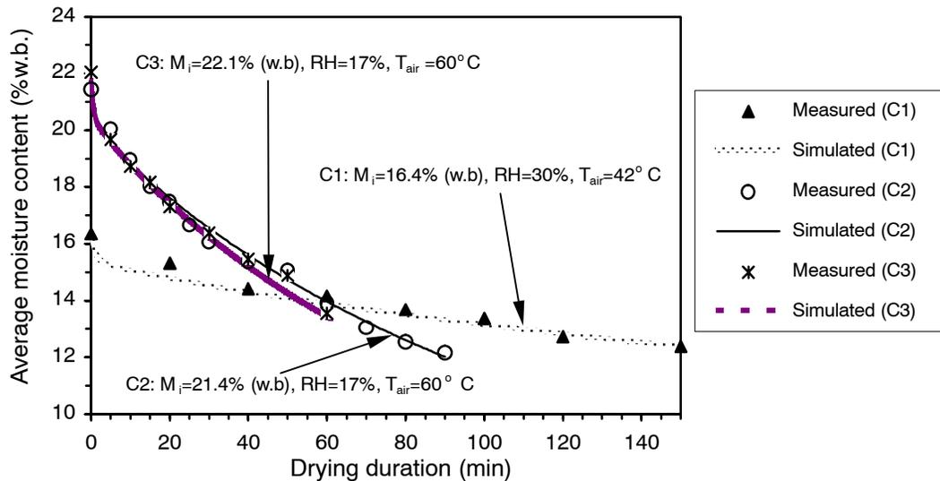
Figure 2. Measured and estimated average moisture contents of rough rice kernels at three thin-layer drying conditions: (C1) 42° C drying air temperature, 30% RH, and 16.4% initial moisture content; (C2) 60° C drying air temperature, 17% RH, and 21.4% initial moisture content; and (C3) 60° C drying air temperature, 17% RH, and 22.1% initial moisture content.
