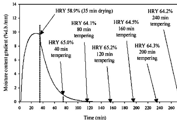
Figure 9. A graph showing the MCGs at 60° C drying air temperature, 17% air relative humidity, and 20.6% w.b. initial moisture content, as well as the head rice yields at the end of drying and at the six tempering durations. Data were based on Clossen et al. (1999). The head rice yield of the control sample was 64.5%.
