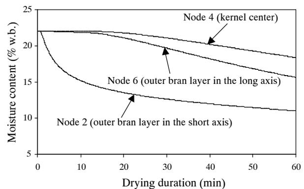
Figure 3. Estimated moisture contents of a rough rice kernel (22.1% w.b. initial moisture content) at three specified nodes at 60° C drying air temperature and 17% air relative humidity.
