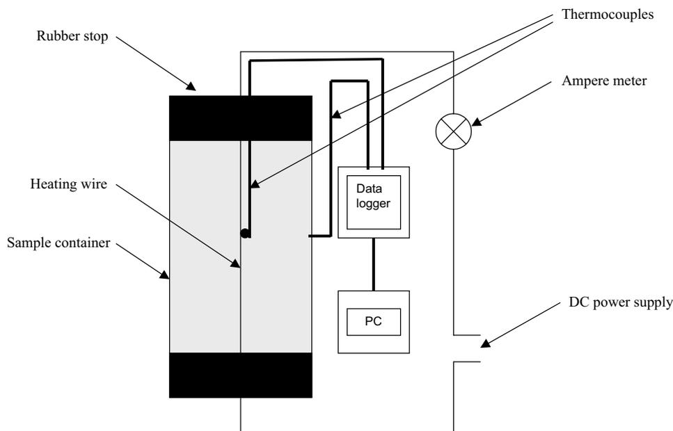
Fig. 1. Schematic of the device for measuring bulk thermal conductivity of rice; PC, personal computer; DC, direct current
