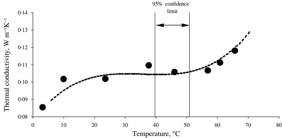
Fig. 4. Mean (●) and Eqn (5) estimated (---) thermal conductivity of Bengal rice at 12.1% initial moisture content (MC) and different initial temperatures; also shown is the 95% confidence limit of the glass transition temperature  $T_g$  for rice by a thermal mechanical analyser at 12.1% MC
