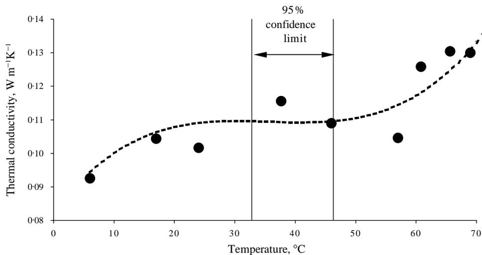
Fig. 5. Mean (●) and Eqn (5) estimated (---) thermal conductivity of Bengal rice at 17.0% initial moisture content (MC) and different initial temperatures; also shown is the 95% confidence limit of the glass transition temperature  $T_g$  for rice by a thermal mechanical analyser at 17.0% MC
