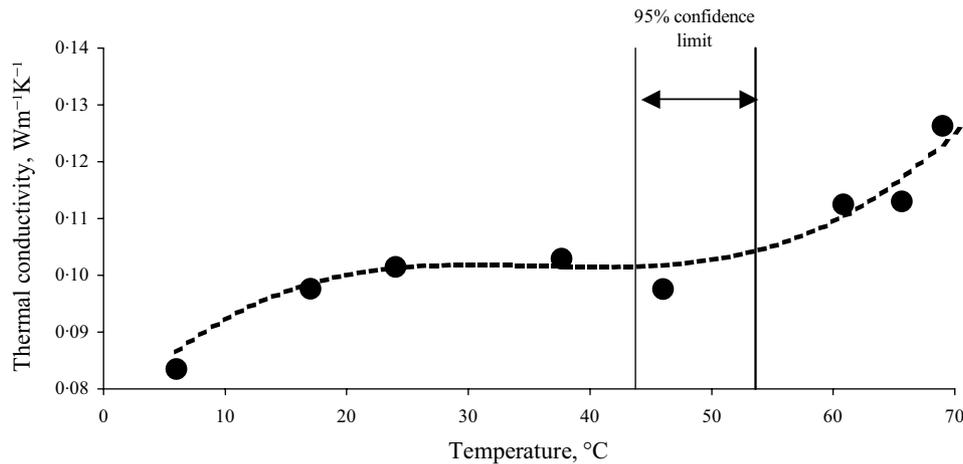
Fig. 3. Mean (●) and Eqn (5) estimated (---) thermal conductivity of Bengal rice at 9.2% initial moisture content (MC) and different initial temperatures; also shown is the 95% confidence limit of the glass transition temperature  $T_g$  for rice by a thermal mechanical analyser at 9.2% MC
