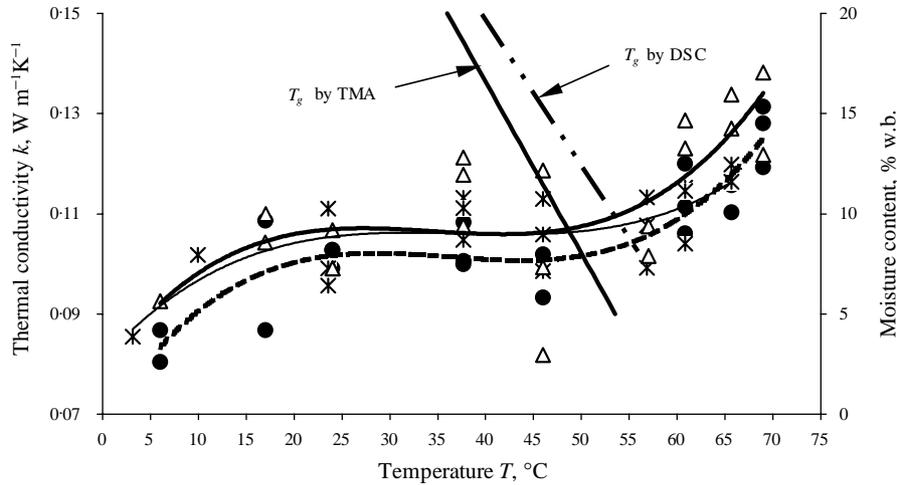
Fig. 2. A combined plot of the rice glass transition state diagrams measured with a thermal mechanical analyser (TMA) (Sun *et al.*, 2001) and a differential scanning calorimeter (DSC) (Perdon, 1999) and the thermal conductivity versus temperature relationships at three moisture contents: 9.2% (● measured, --- estimated), 12.1% (\* measured, — estimated) and 17.0% (Δ measured, — estimated)
