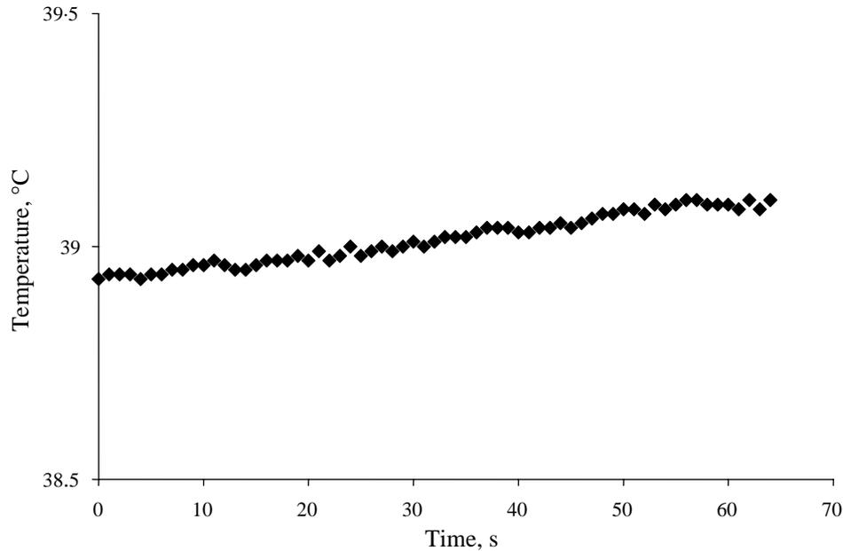
Fig. 6. The surface temperature of the sample holder as a function of time during one measurement at an initial temperature around 39°C
